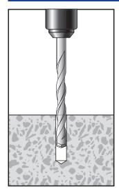
Using the proper diameter bit, drill a hole into the base material to a depth of at least 13mm or one anchor diameter deeper than the embedment required.
