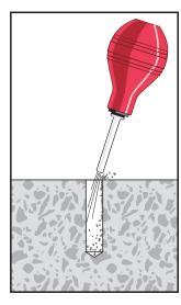
Blow the hole clean of dust and other material. Do not expand the anchor prior to installation
