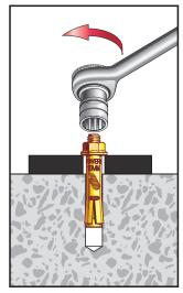
Tighten the anchor by turning the head 3 to 4 turns or by applying the guide installation torque from the finger tight position.
