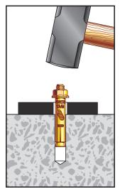
Drive the anchor through the fixture into the anchor hole until the head is firmly seated against the fixture. Be sure the anchor is driven to the required embedment depth.
